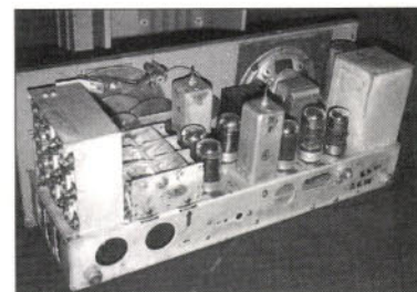
Fig. 3: The inside of the R-103 Mark 1. The coil pack and tuning components are on the left of the picture, with the i.f. stages in the middle. The vibrator power pack is mounted on the right hand side of the chassis.
