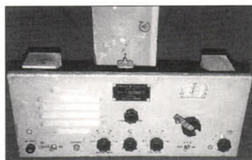
Fig. 2: The R-103 Mark 1 Canadian. Note the built-in speaker on the left, with main tuning knob on the right.
